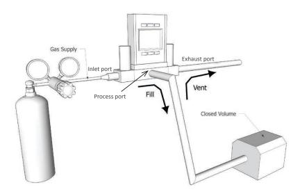
Fig. 2 Typical EPR Plumbing Diagram
